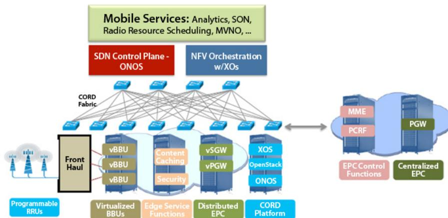
Figure 2 – M-CORD RAN Network Slicing Virtualization
