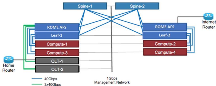
Figure 5 - R-CORD Access Rack Hardware
