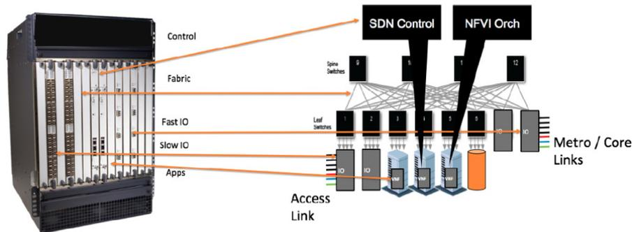
Figure 4- Disaggregating OLT
