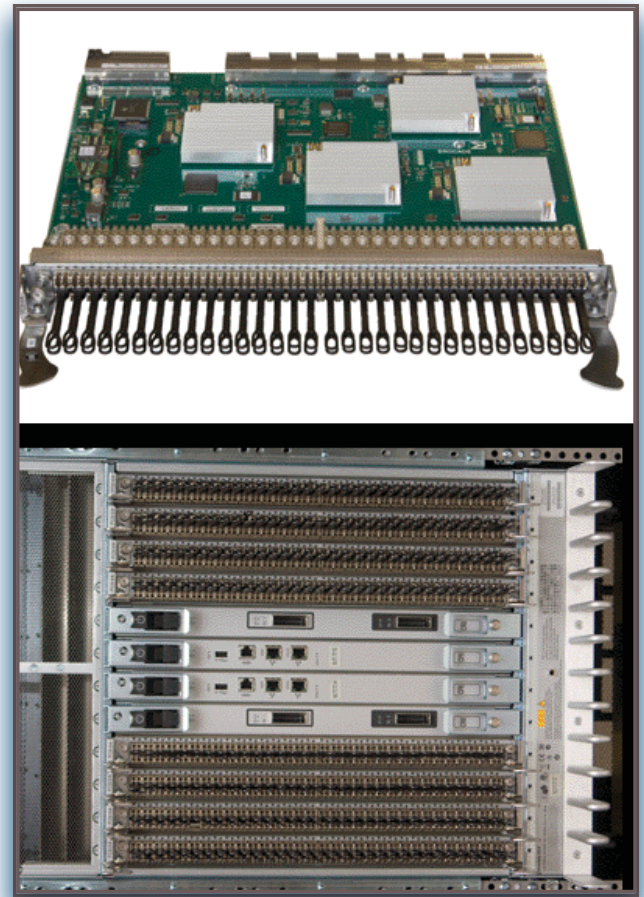
figure 2: Brocade Fibre Channel blade (top) and DCX Chassis (bottom)
