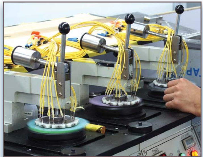
figure 6: Fiber optic connectors being polished at our facility
