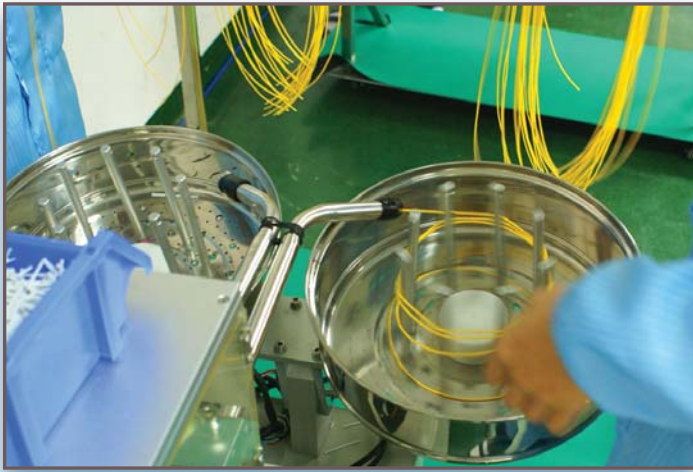
figure 2: Automated cut/coiling unit
