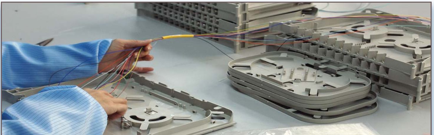
figure 3: Technican assembling fiber optic spice trays
